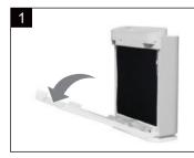
Place your fingers in the recesses of the side panels and gently pull the top part of the front panel towards you. Then, lift the hooks at the bottom of the panel out of the bottom of the unit.
