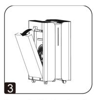
Remove the filters from the unit.
