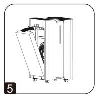
Reinsert the filters into the unit.
